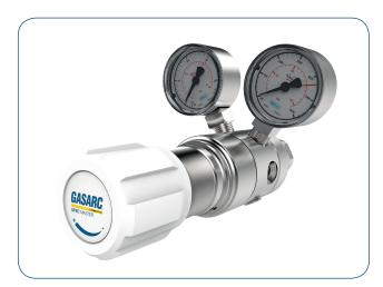
The Spec Master HPT620 Series two stage piston cylinder regulators are designed for primary pressure gas control of non-corrosive or toxic, high purity gases up to grade 6.0 purity (99.9999%), on applications where constant delivery pressure is required as the cylinder pressure decreases.
