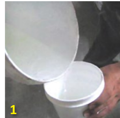
1 Add 1 litre of T-007 & 3 litres water to mix container.
