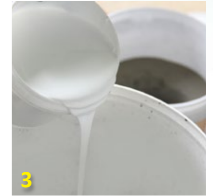
3 Add resin (part A) to a empty pail. Add 0.7kg clean water to mix container.
