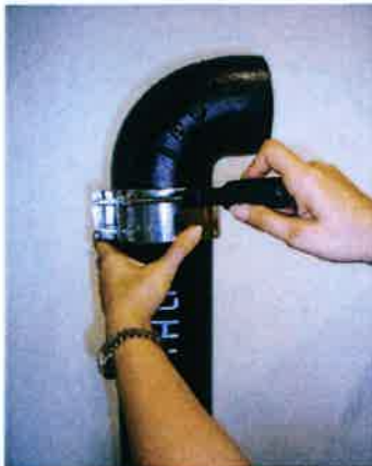
3. Insert the fittings spigot into the rubber gasket.
