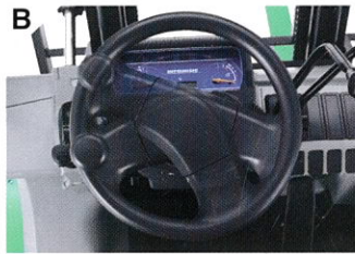
B Power Steering With 100% Standstill Steering
