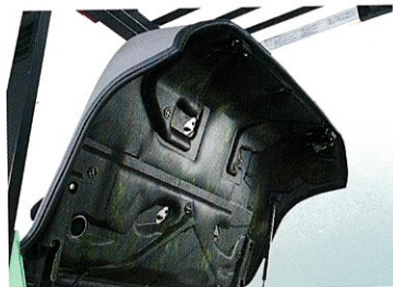
Quality foam inside the engine cover as noise absorber.
