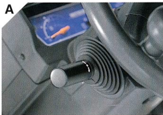
A Electric FNR Lever (Automatic Transmission Models)
