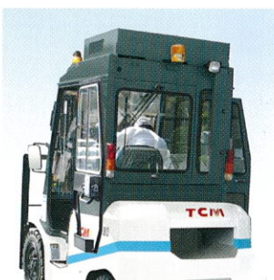
Steel cabin-enclosed type with air-cooler (available for 2-3.5ton models)
