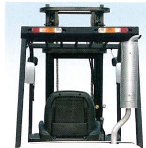
Overhead exhaust system
