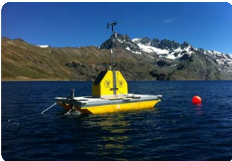
Monitoring Buoy containing a YSI Sonde, and meteorological sensors.
