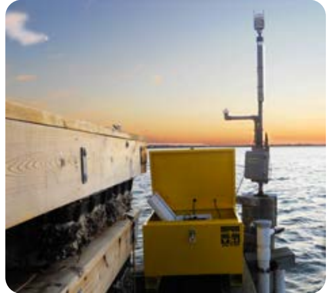
Portable aluminum chest monitoring system containing a YSI Bubbler, Sonde, Data Logger, and meteorological sensors.
