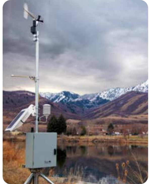
Monitoring station containing a YSI Storm 3 Data Logger, and meteorological sensors.
