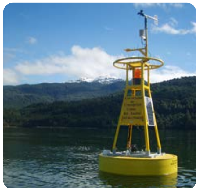
Monitoring Buoy containing meteorological sensors.
