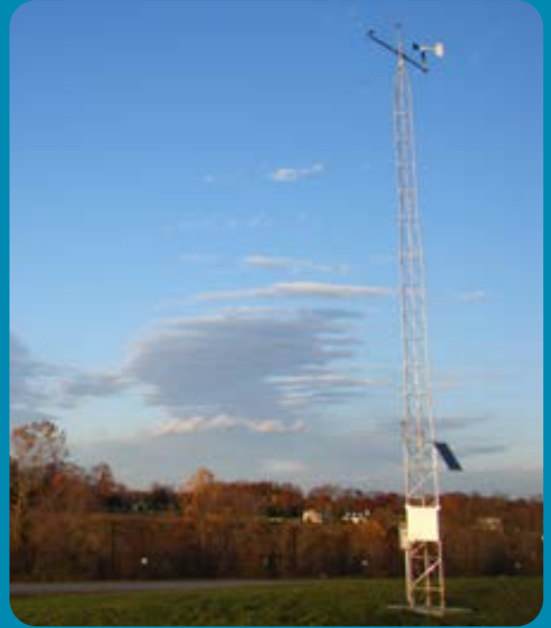
10 meter monitoring tower containing meteorological sensors, data logger, and cellular telemetry.
