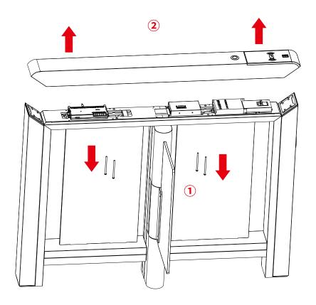
$3. \quad \ \mbox{Remove the side lid that hang on the device.}$
