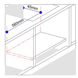
The panels of the adjacent cabinets must be made of heat resistant material. In particular, cabinets with a veneer exterior must be assembled with glues which can withstand temperature of up to  $100\ \mathrm{C}$
