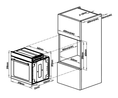
In order to ensure adequate ventilation, the back panel of the cabinet unit must be removed. Installing the oven so that it rests on two strips of wood is preferable. If the oven rests on a continuous, flat surface, there must be an aperture of at least 45x560mm.
