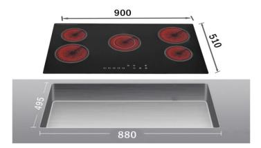
Create an opening with the dimensions shown in the paragraph 10.1 in the top surface of the counter, keeping a minimum distance of 50mm from the rear edge.
