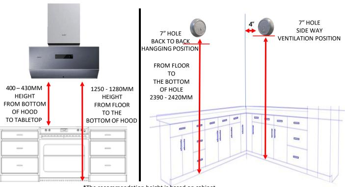
\*The recommendation height is based on cabinet height 850mm.
