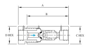
BuTech o-ring check valves reliably prevent backflow where leak-tight shutoff for liquids or gases is required. Standard materials of construction are 316 stainless steel with Buna-N o-ring and 300 series stainless steel spring.
