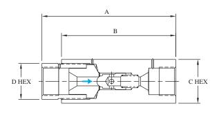
BuTech ball check valves prevent reverse flow where leak-tight shutoff is not necessary. Standard materials of construction are 316 stainless steel with 17-4PH poppet for longer life, and 300 series stainless steel spring.
