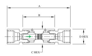
BuTech line filters are used in system lines to remove contaminating particles from the system fluid. Upstream filter of larger micron rating than downstream filter to prevent clogging of downstream filter.
