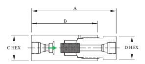
BuTech sintered cup filters offer maximum filtration surface area for removal of contaminating particles from the fluid system. They may be used in systems which require high flow rates with minimum pressure drop.
