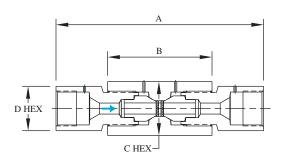
BuTech line filters are used in system lines to remove contaminating particles from the system fluid. Upstream filter of larger micron rating than downstream filter to prevent clogging of downstream filter.
