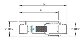
BuTech sintered cup filters offer maximum filtration surface area for removal of contaminating particles from the fluid system. They may be used in systems which require high flow rates with minimum pressure drop.
