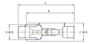
BuTech ball check valves prevent reverse flow where leak-tight shutoff is not necessary. Standard materials of construction are 316 stainless steel with 17-4PH poppet for longer life, and 300 series stainless steel spring.
