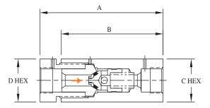
Cracking pressure: 15 PSI (1 bar) approximate Operating Temperature Ranges:
