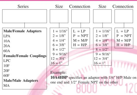
BuTech offers a complete line of adapters and couplings manufactured from 316 cold-worked stainless steel. Pressure gauges, thermocouples and high-pressure hose are also available to complete your system.
