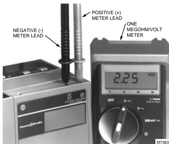
Fig. 22. Flame signal measurement.
