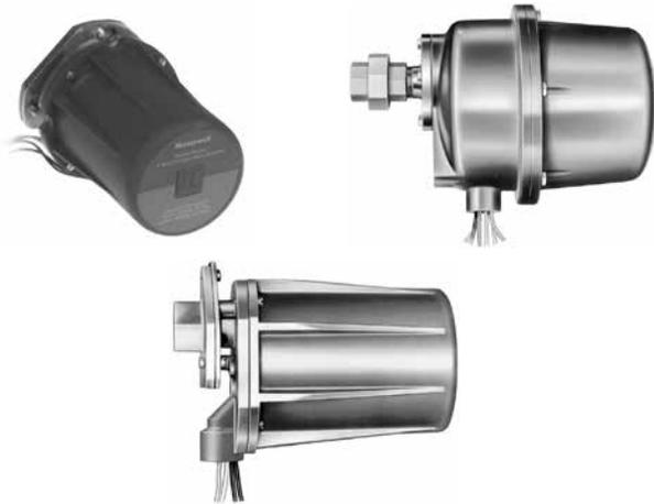
**Solid state electronic flame detectors for use with Honeywell Flame Safeguard controls and amplifiers. Sense ultraviolet radiation produced by combustion of gas, oil, coal or other fuels.**
