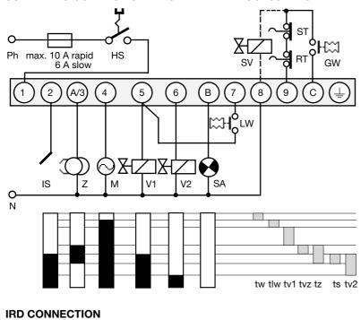
ST Limit thermostat Control thermostat RT IS Ionization probe Ignition Ζ Μ Burner motor V1 Solenoid valve 1st stage V2 Solenoid valve 2nd stage LW Air pressure monitor External fault indication SA SV Safety valve Waiting time at start-up tw Max. reaction time tlw for air proving switch tv1 Pre-purge time Pre-ignition time tvz tz Total ignition time Safety time ts tv2 Time delay term.6 / term.C
