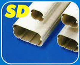
SLIMDUCT SD Composed of bottom section and upper section(cover). They can be installed very simply by first fixing bottom section to the wall, then setting the pipes and wires and lastly putting the cover.
