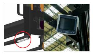
A fork camera is installed on the truck to improve safety and
