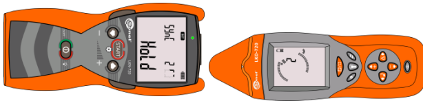
Fig. 5 Positioning the transmitter and receiver during synchronization
