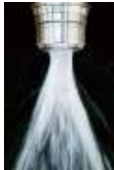
Flood Jet-Through Coolant
