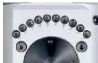
Indexing mechanism in 1° increments
