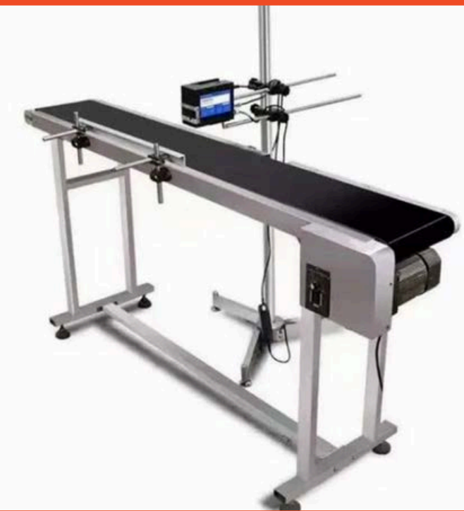
Inkjet printing Machine Print the Manufacturing Date in the can
