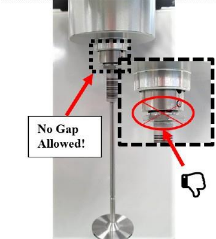
Figure III-2.4: Gap, Not Correct
