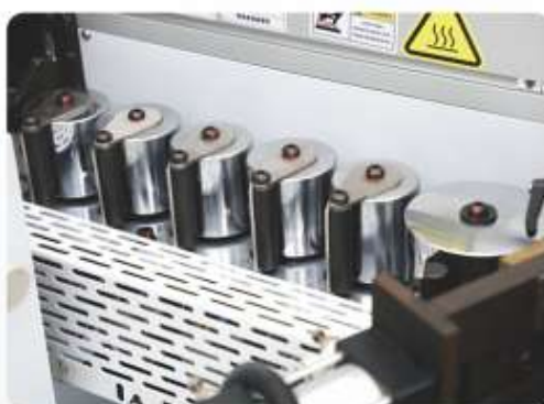
六轮压贴 Six-wheel pressing
