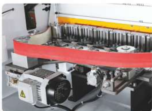
履带压贴 Crawler pressing
