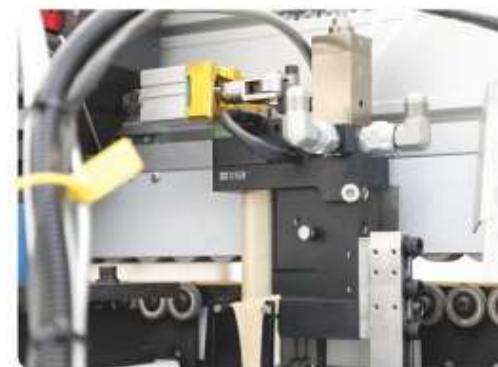
PUR免清洗胶锅 PUR no-clean glue pot
