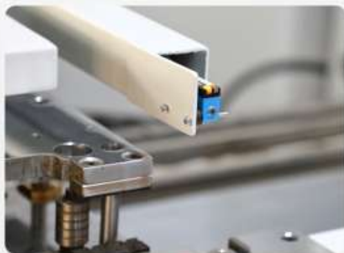
板材尺寸光电自动识别 Panel size photoelectric automatic identification
