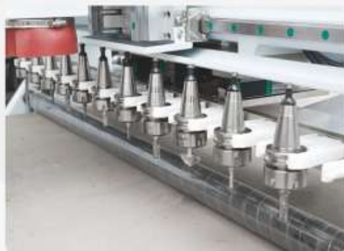
12直排刀库 12 linear tool magazine
