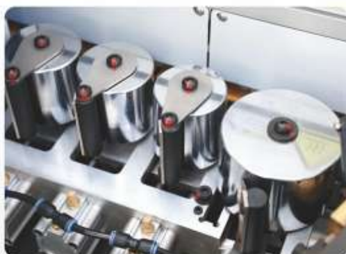
四轮压贴 Four-wheel pressing
