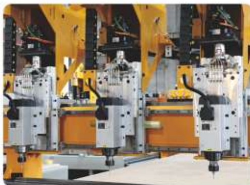
分体式三独立主轴加工 Split-type three independent spindle machining
