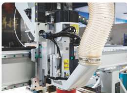
9kw风冷自动换刀主轴加工 9kw air-cooled automatic tool changer spindle machining
