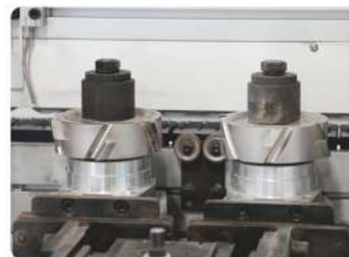
板材边缘预铣 Pre-milling of board edges
