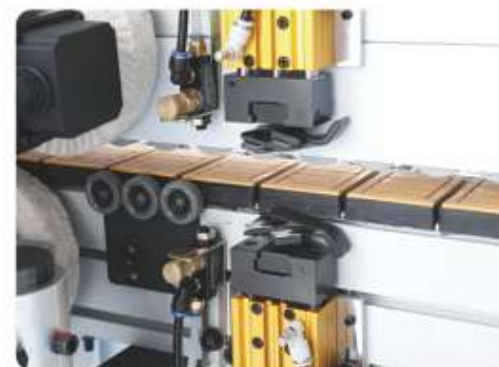
柔性平刮 Flexible scraping
