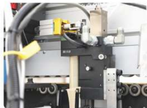
PUR免清洗胶锅 PUR no-clean glue pot
