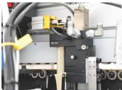
PUR免清洗胶锅 PUR no-clean glue pot
