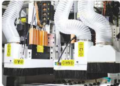
抗震变频上钻组 Anti-seismic variable frequency top drill unit
