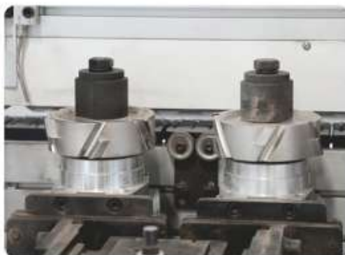
板材边缘预铣 Pre-milling of board edges
