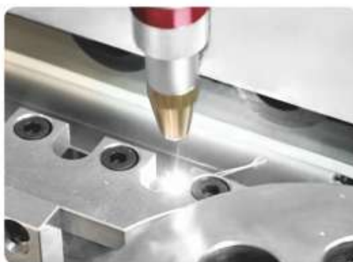
激光焊接封边 Laser welding edge sealing
