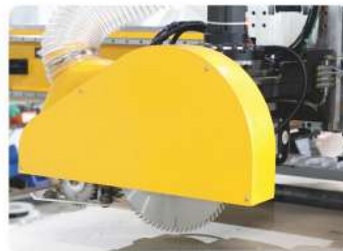
子母锯片可 \pm 90^\circ 度旋转加工 Large and small saw blades can rotate \pm 90 degrees for processing
