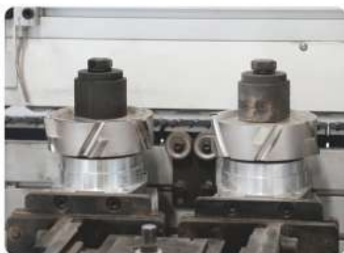
板材边缘预铣 Pre-milling of board edges
