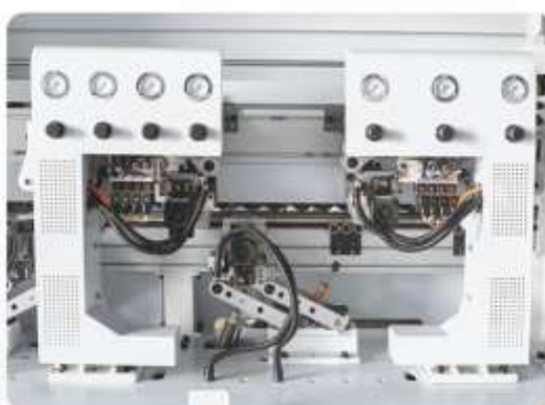
四电机高速跟踪 Four motors high-speed corner rounding
