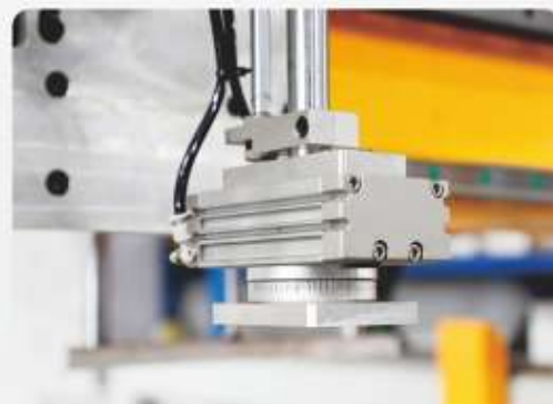
\pm 90^\circ 度旋转贴标装置 (连线配置) \pm 90 degree rotating labeling device (connection configuration)
