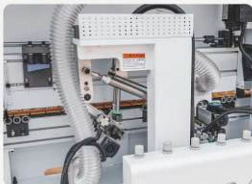
双电机跟踪 Double motors corner rounding
