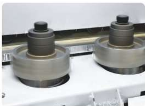
板材边缘预铣 Pre-milling of board edges
