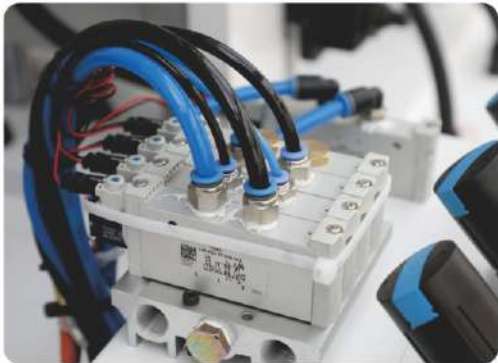
电磁阀配置费斯托 (KE-500H/356) Festo solenoid valve configuration (KE-500H/356)
