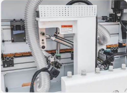
双电机跟踪 Double motors corner rounding
