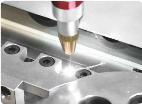
激光焊接封边 Laser welding edge sealing
