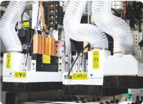
抗震变频上钻组 Anti-seismic variable frequency top drill unit
