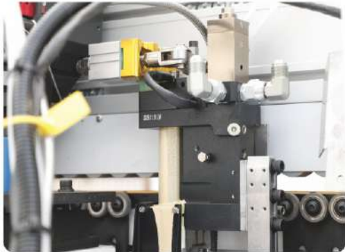
PUR免清洗胶锅 PUR no-clean glue pot
