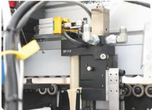
PUR免清洗胶锅 PUR no-clean glue pot
