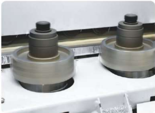
板材边缘预铣 Pre-milling of board edges
