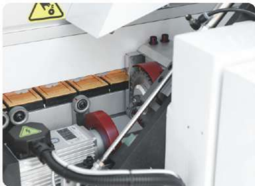
单导轨齐头 Single rail end cutting
