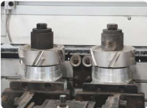
板材边缘预铣 Pre-milling of board edges
