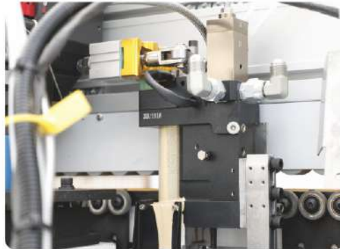
PUR免清洗胶锅 PUR no-clean glue pot
