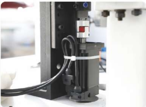
送带/压贴伺服控制 Servo control for edge band feeding and pressing
