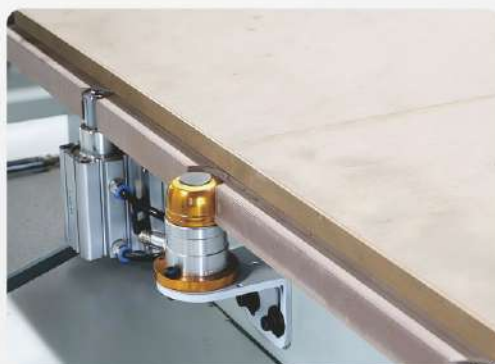
高精度对刀仪 High-precision tool setting instrument
