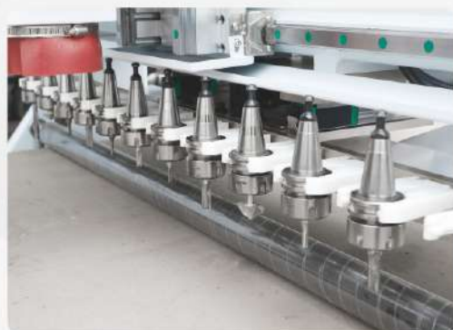
12直排刀库 12 linear tool magazine
