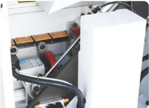
单导轨齐头 Single rail end cutting
