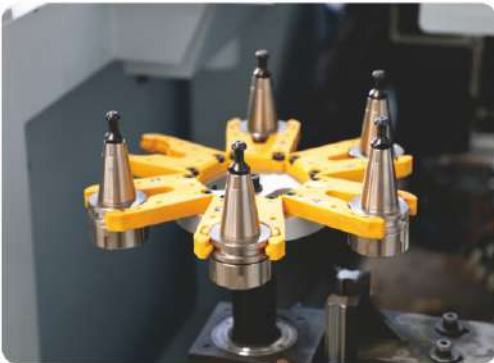
六刀库自动换刀 Six tool magazines automatic tool change
