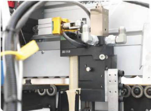
PUR免清洗胶锅 PUR no-clean glue pot
