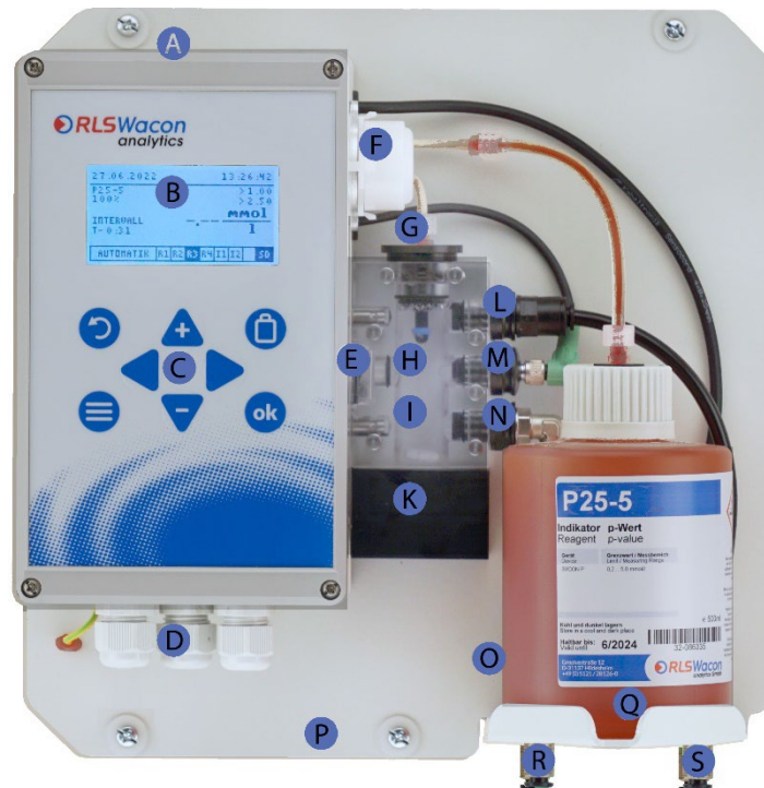
Figure 22: SYCON P analyser with inserted reagent bottle
