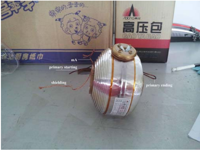
High voltage coil
