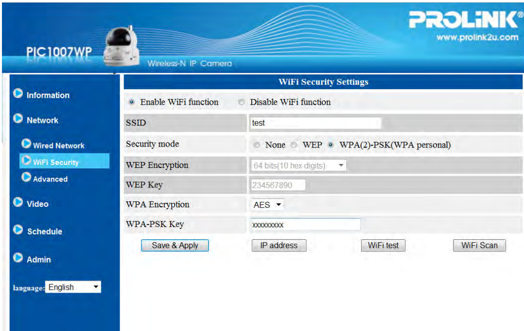
Figure 3-8: WiFi security enabled page
