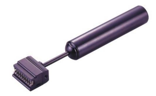
This 5-Pair 110 Punchdown Tool from DINTEK offers a quick solution when needing to punch down large groups of cables. For use on LAN and Telecom cables with seating of 4 or 5 pairs at a time. Suitable for both 110 type cable side and cross-connect side terminals blocks. The termination block heel w/blades are changeable and reversible. One end for seating and cutting off wires, and the other end for seating wires only.
