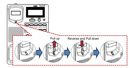
5. If you wish to temporarily place the handset down during a conversation, hook the handset onto the top of the hanger hook as shown below.
