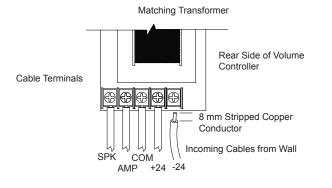
Cables from amplifier, to speakers and the overriding 24V DC shall be connected to the module before mounting to the back enclosures.
