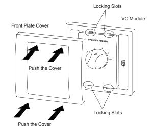
The final procedure shall be attaching the front plate cover to the VC assembly. Gently push the cover with the locking pin to the slots to complete the installation
