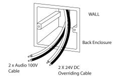
As the volume controllers works in a 4 wire system, there should be 2 x 100V line audio circuit from power amplifiers and another optional 2x24V DC emergency overriding cable from the rack.
