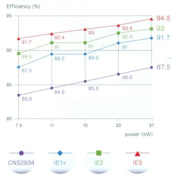
CNS2934 is the standard of old version for 3-phase squirrel cage induction motor.
